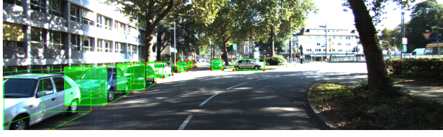
Fig. 3. Some qualitative 3D detection results on the KITTI test set.
